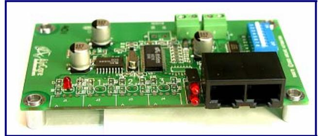
For use with the ACC1 or ACC2 series consoles, ACM1009 requires a DIP Switch address of 253 (FD hex), shown below.
