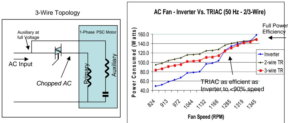
Figure 2: 3-Wire Topology & Improved Power Consumption Data
