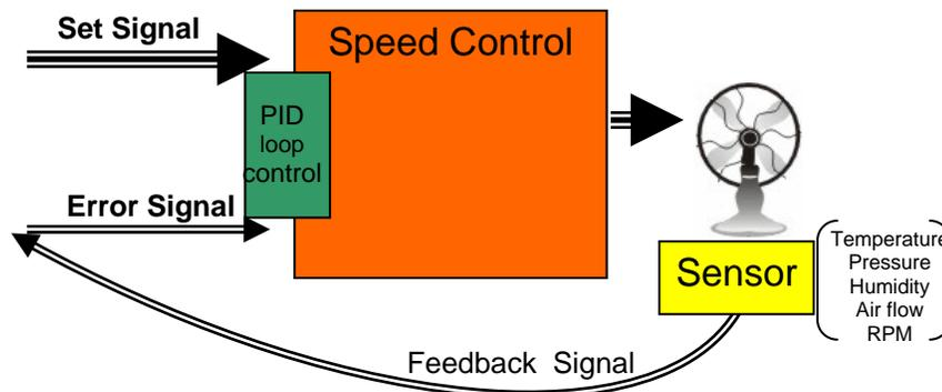
**Figure 6: Close Loop Control Using External Sensors**
