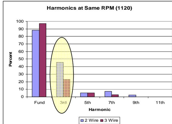
**Figure 3: Harmonic Distortion for identical fan running at reduced speed**
