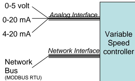
**Figure 5: Interface Control – Analog, Network or “other”**
